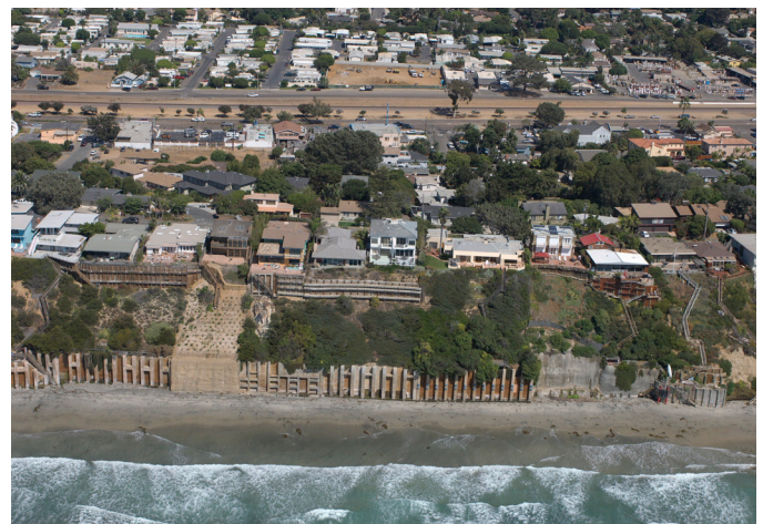
Figure 5.2 Most of the developed cliffs of the city of Encinitas have now been armored (Kenneth and Gabrielle Adelman, California Coastal Records Project).
