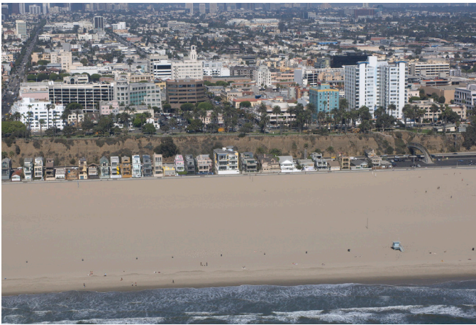
Figure 3.23. Wide sandy beach provides a buffer to the backing bluff from wave attack and it will require a significant rise in sea level before such areas are exposed to direct wave attack (Kenneth and Gabrielle Adelman, California Coastal Records Project).
