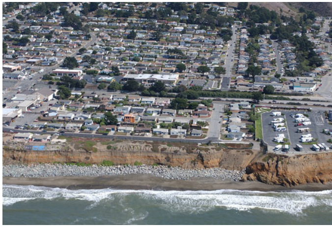
Figure 3.20. Bluff retreat in Pacifica during the 1997-1998 El Niño led to the loss of an entire row of oceanfront homes (Kenneth and Gabrielle Adelman, California Coastal Records Project).
